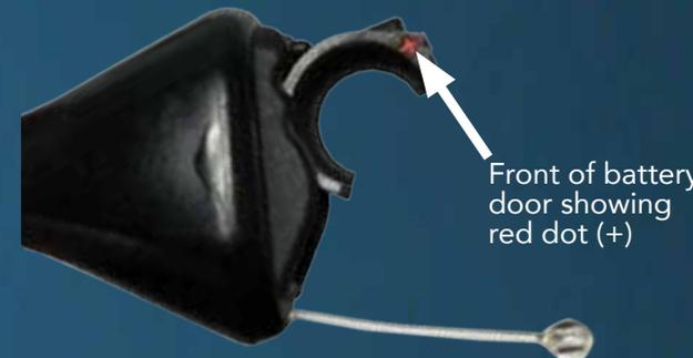
**Note:** The domed side of the battery is negative and the completely flat side is positive. The flat side (+) needs to be on the red dot door (+) side.
